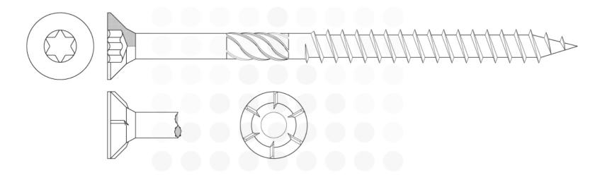
TORX RECESS COUNTERSUNK FLAT HEAD WITH 6 NIBS UNDER HEAD TWIN THREAD AND PARTIAL THREAD WITH SERRATION HEAD
